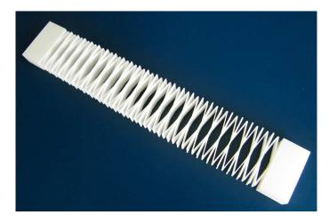
Fig. 10: Prototype of the final version of the accordion honeycomb core [21].
