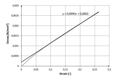
Fig. 11: Stress-strain curve of the accordion honeycomb core [21].
