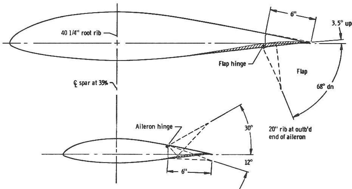
Wing profiles with cross hatched areas showing HP-14 modification of basic FX 61-163 airfoil and flap and aileron detail
