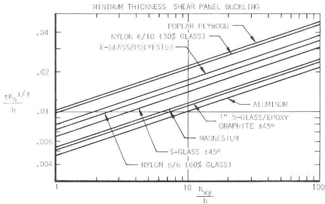
Shear buckling:  $\tau_{cr} = \frac{K_s E_c t^2}{b^2}$
