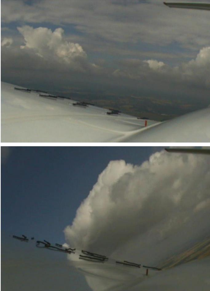
**Figure 18** VSO10C sailplane, wing root tuft visualization,  $V = 140$  km/h IAS, attached flow (top);  $V = 70$  km/h IAS, bank angle 30 deg, stalled flow (bottom).
