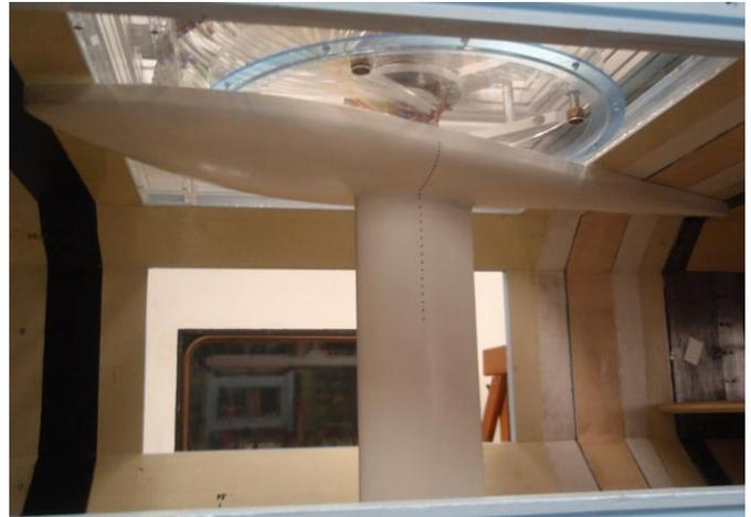
**Figure 5** T10 test case geometry in the test section 865 x 485 x 900 mm<sup>3</sup> wind-tunnel of the IT, AS of the CR with side walls removed.
