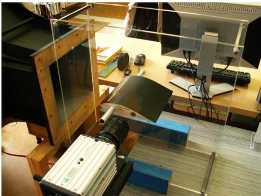
**Figure 4** Blow-down rig of 250 x 250 mm<sup>2</sup> of the IT, AS of the CR and time-resolved PIV setup with Wortmann FX66-S196V1 airfoil.
