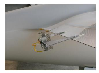
**Figure 7** Installation of pressure rake downstream the HPH304S wing trailing edge.
