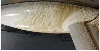
Figure 19 Oil-flow visualization in 750 x 550 mm<sup>2</sup> wind tunnel test section on T10 test case 1:5 scale model,  $Re_c = 2.0 \times 10^5$ ,  $\alpha = -5 \text{deg}$ .
