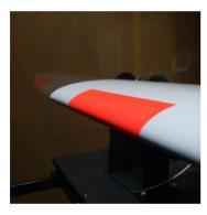
Figure 3 VSO10 wing segment with end plates with simulated strip of roughness due to insects in the  $750 \times 550 \text{ mm}^2$  wind-tunnel CTU in Prague.
