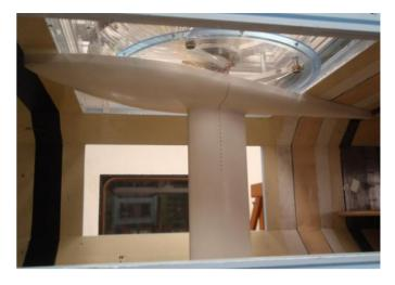
**Figure 5** T10 test case geometry in the test section  $865 \times 485 \times 900 \text{ mm}^3$  wind-tunnel of the IT, AS of the CR with side walls removed.
