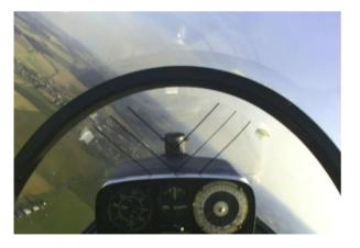
**Figure 10** Still image from in-flight video recording, VSO10C sailplane, V = 80 km/h IAS, note lines on transparent film as a reference for turn reversal from -45 deg to +45 deg bank.
