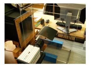
**Figure 4** Blow-down rig of  $250 \times 250 \text{ mm}^2$  of the IT, AS of the CR and time-resolved PIV setup with Wortmann FX66-S196V1 airfoil.
