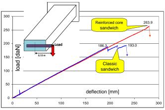
Figure 16 Load versus deflection of both specimens.
