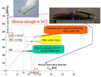
**Figure 1** Example of the advisory chart regarding composite wing spar with GFRP spar flanges and GFRP shear-web.<sup>1</sup>
