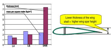
Figure 8 Mass and thickness of some chosen plates.
