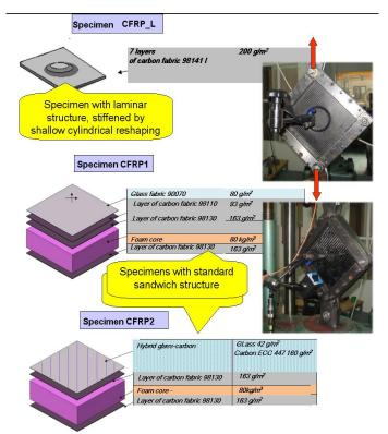
**Figure 10** Specimen of shell with laminar structure, stiffened by shallow cylindrical reshaping and specimens with standard sandwich structure.
