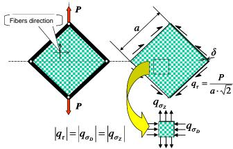
Figure 3 The loads of the specimen structure.
