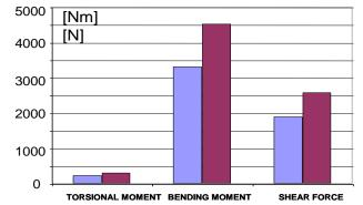
Figure 17 Comparison between particular loads in the roots of beam boxes.
