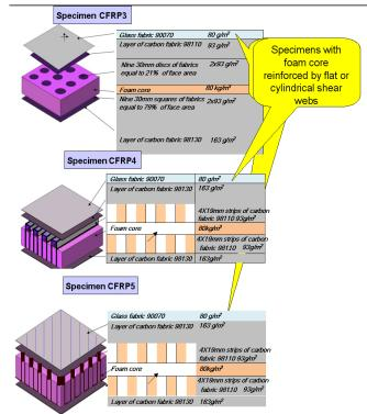
Figure 11 Specimens with foam core reinforced by flat or cylindrical shear webs.
