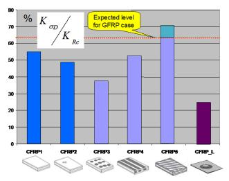
Figure 13 Loading abilities of different CFRP shells subjected to shear loading.
