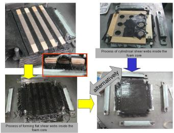
Figure 12 Methods of foam core reinforcement.
