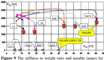
different shells (dashed lines mean extrapolation up to failure load).
