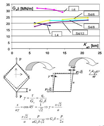
Figure 7 Comparison of shear stiffness and principle of  $G\delta$  value estimation.
