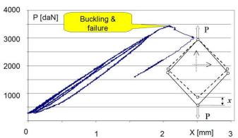
Figure 6 Behavior of the shell subjected to shear loads with increasing amplitude.
