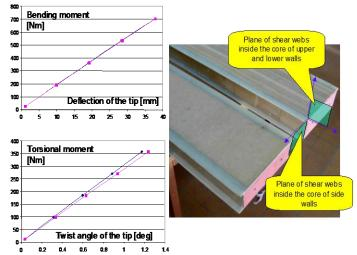
Figure 15 Comparison of specimen stiffness.
