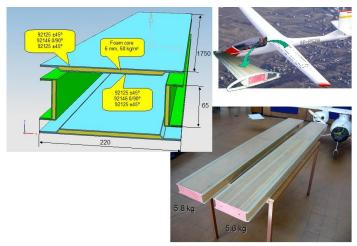
Figure 14 Shape and weight of the specimens for comprehensive testing.
