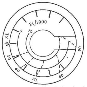
FIGURE 1. A modified MacCready ring calibrated for heights of sea-level, 5,000 ft and 10,000 ft. The markings are on a clear plastic disc attached to the usual verge ring. Variometer details have been omitted for clarity. Speeds are in knots and the calibration applies to the maker's polar for the "Standard Libelle."
