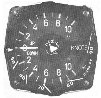
FIGURE 2. Perhaps a more practical arrangement. The inner edge of the verge ring is calibrated for sea-level, the outer edge for 10,000 ft. Approximate interpolation for other heights should be good enough. The calibration is for the "Standard Libelle."  $(dH/dt)_{indicated} = (dH/dt)_{true} \times \sigma^{\eta}$  (1)
