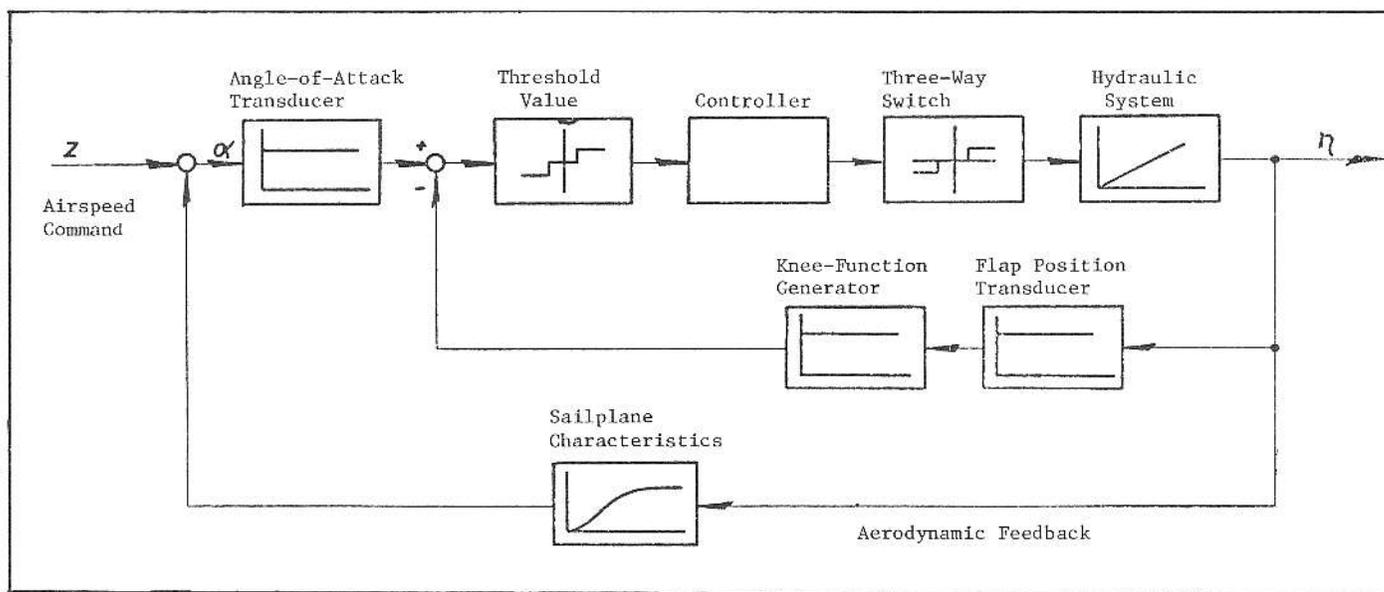
FIGURE 4. Block Diagram of Automatic Flap Control System
