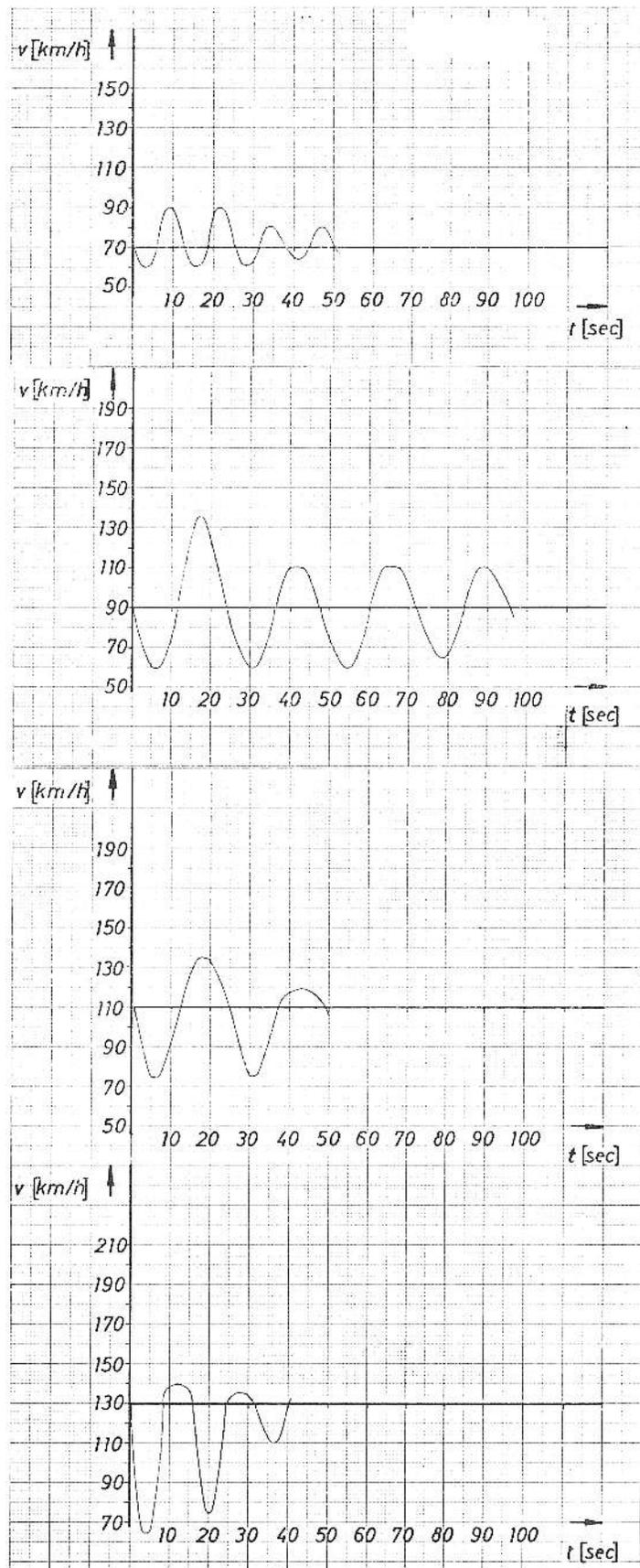
FIGURE 9. Stick-Fixed Speed/Pitch Characteristics of Sailplane under Automatic Flap Control
