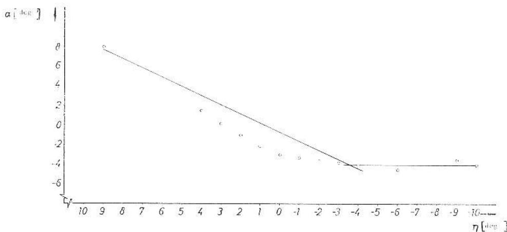
FIGURE 3. Approximation to the Relation Between Optimum Flap Angle and Angle-of-Attack Using Two Straight Lines.
