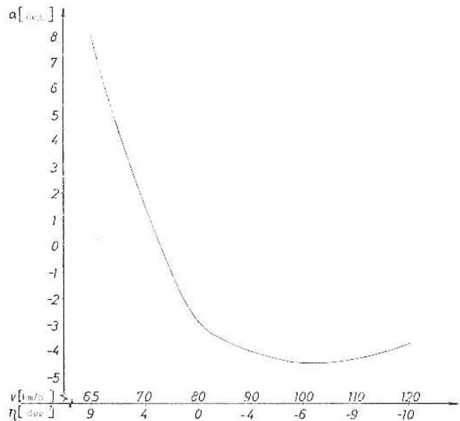
FIGURE 2. Indicated Angle-of-Attack as a Function of Airspeed and Flap Angle as Measured Using Wool Tuft at Station 7.
