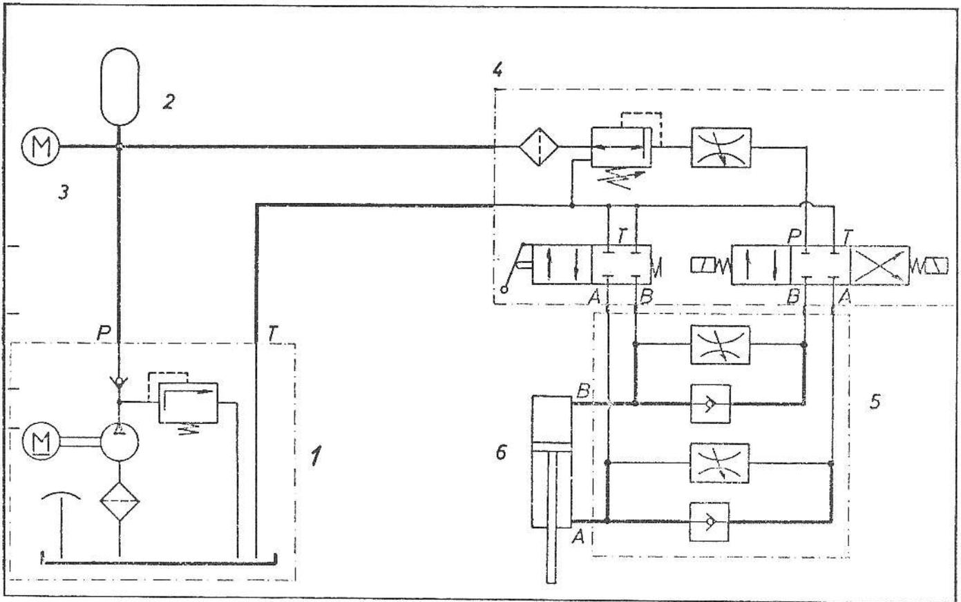
FIGURE 5. Block Diagram of the Hydraulic System
