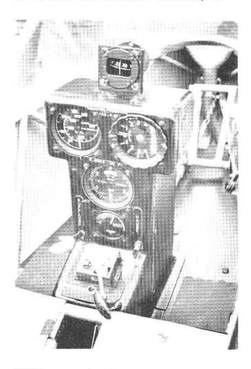
FIGURE 8. Hydraulic System Installation in "Baggage Space."
