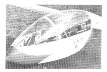
FIGURE 6. Angle-of-Attack Measuring Vane Installed on Side of Cockpit.
