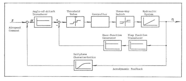
FIGURE 4. Block Diagram of Automatic Flap Control System
