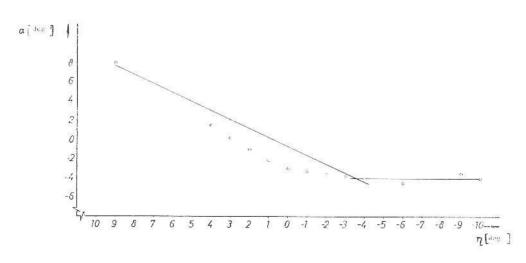
FIGURE 3. Approximation to the Relation Between Optimum Flap Angle and Angle-of-Attack Using Two Straight Lines.
