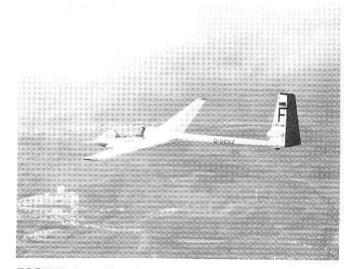
FIGURE 1. FK-3 Sailplane with Full-Span Camber-Changing Flaps/Ailerons.
