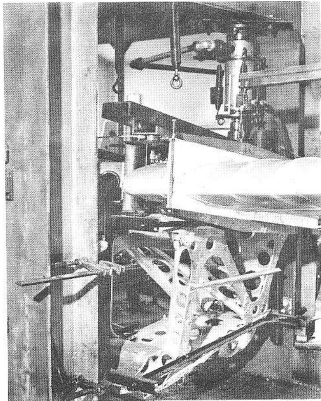
Figures 11 and 12. Gobe fatigue test.
