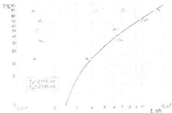
Figure 9. Fatigue Life Distribution in Normal Hours.
