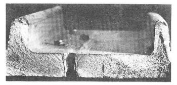
Figure 4. Main Spar Boom Failure at the Diagonal Junction.
