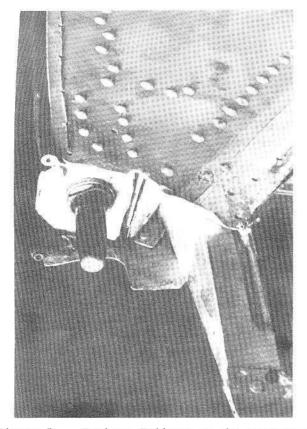
Figure 5. Fatigue Failure at the Rear Wing Attachment Bold.
