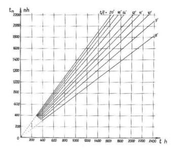
Figure 10. Conversion of Flying Hours into Normal Hours.
