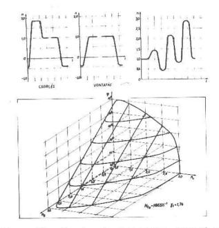
Figure 2b. Service Load Spectra: Ground to Air Cycles, Spinning, Thermalling.
