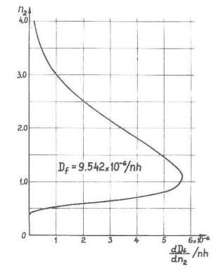
Figure 7. Damage Curve for Start and Landing.
