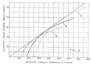
Fig. 2 (curve A) shows a plot of achieved cross-country speed against absolute thermal strength. The absolute thermal strength has been obtained by adding 1.5×minimum sinking speed to the achieved rate-of-climb. The value of 1.5 is purely arbitrary and is my guess of a likely value of achieved sink relative to the air when thermalling.
