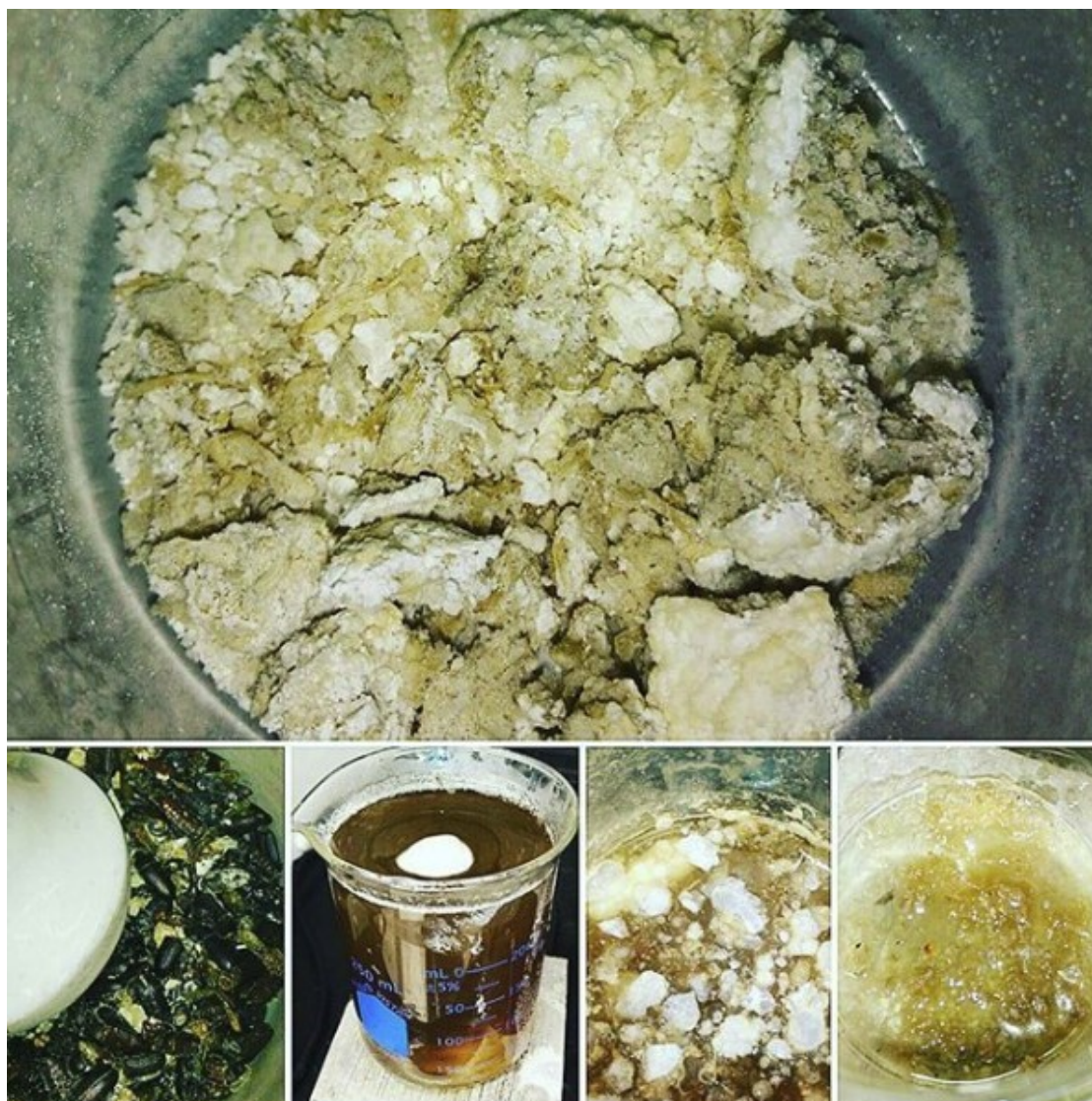
Figure 2: A chitosan based plastic substitute made from T. molitor beetle shells. On Top: The finished biodegradable plastic substitute. On Bottom, from left to right. a) Breaking down T. molitor beetle shells by grinding. b) Removal of organic matter. c) Deprotonation of T. molitor beetle shells. d) Evaporating excess liquid to form chitosan sheets.
