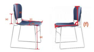
**Figure 1:** Visual representation of: (a) Chair Seat Height, (b) Chair Seat Pan Width, (c) Chair Seat Pan Length, (d) Chair Backrest Height, (e) Chair Lumbar Support Height, (f) Chair Angle.
