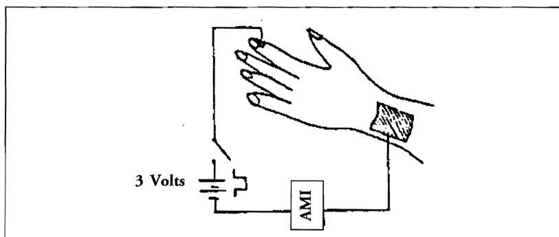
**Figure 2.** Placement of electrodes, AMI instrument.
