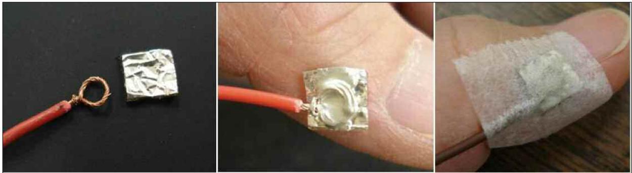
Figure 3. (left) Gel electrode and Lead Wire, (middle) Lead wire bonded to Gel electrode with Conductive Adhesive, (right) Electrode securely attached to Jing-Well point.
