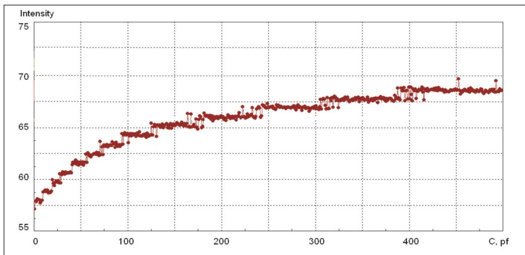
people present, variability of data during 6 hours remained at the level of 0.5–1%. Before collecting field data, the measurement instrument should be “warmed up” by operating for 30-50 minutes with the cylinder connected to the grounding jack of the instrument, rather than being connected to the antenna.
