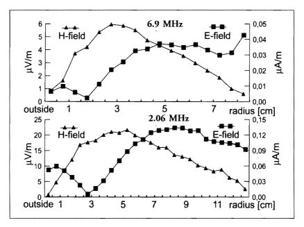
**Figure 2.** Top: The electric and magnetic field in dependence of the radius (cm) of the Tesla coils generating longitudinal waves at  $6.9 \pm 0.1$  MHz. Bottom: The electric and magnetic field in dependence of the radius (cm) of the Tesla coils generating longitudinal waves at 2.06  $\pm$  MHz.
