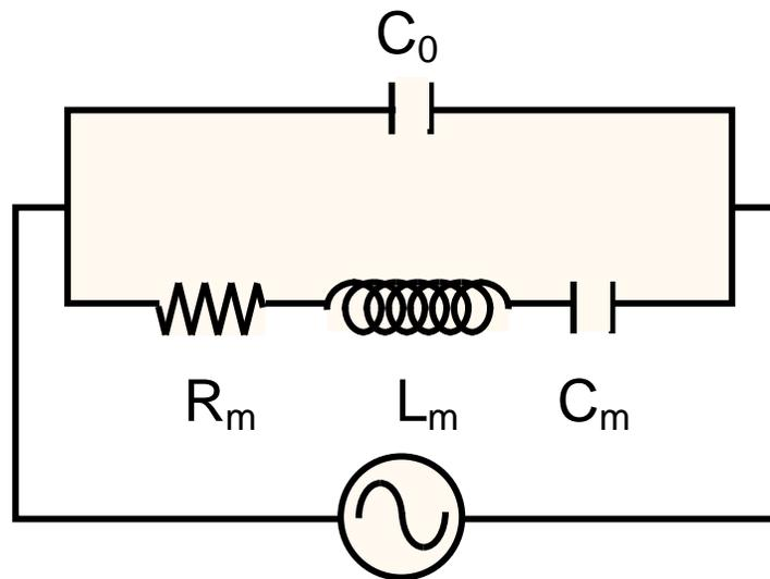
Figure 4. The electrical model of the liquid interface
