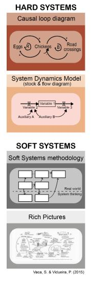
the stock and flow diagrams. This is the way that system dynamics models are built and also the tool used to work and communicate relationships and concepts represented by the model through shapes, figures and letters. The basic structure of stock and flow diagrams is showed on figure 2.
