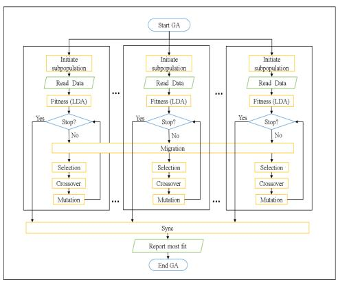
Figure 4. High-Performance GA-LDA Structure
