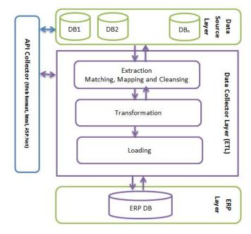
Figure 2. Abstracted Solution Architecture
