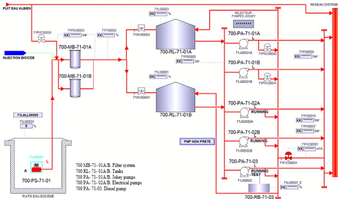
Figure 3. Simplified flow diagram of the fire-fighting systems of the liquefied petroleum gas storage.
