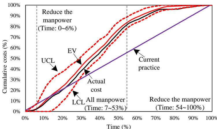
Figure 7. Overall project budget percentages and cost control limits for the test case.
