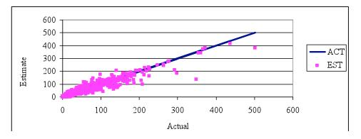
Figure 4. Neural Network Estimate with 8 Variables vs. Actual Concrete Shear Strength
