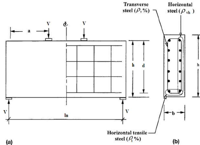
Figure 1. Basic Parameter for Deep Beam Model a) elevation b) Cross-Section (adapted from Sanad and Saka, 2001)
