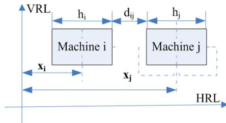
**Figure 3. The variables of the layout in one line model**
