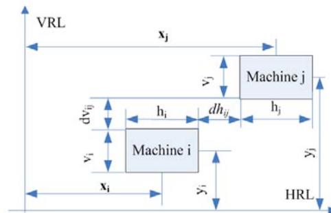
**Figure 4. The variables of the layout in multi-line model**
