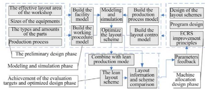
**Figure 2. Design process of the system**
