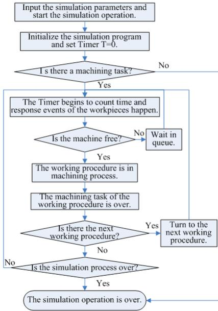
Figure 5. Simulation flowchart of the layout system
