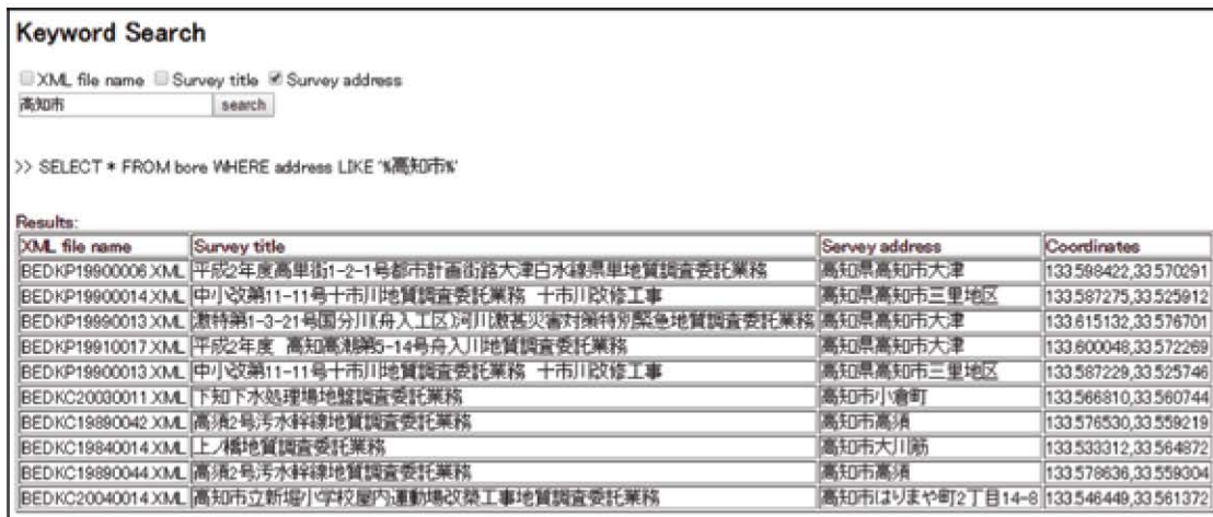
Figure 8. Results of a keyword search. First five in results were obtained from the database for Kochi Prefecture's data, and the rest were obtained from the database for Kochi City's data
