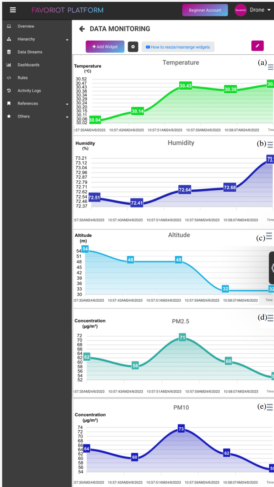
Figure 8: The User Interface (UI) and the dashboard of the IoT platform (a) temperature (b) humidity (c) altitude (d) PM 2.5 concentration (e) PM 10 concentration
