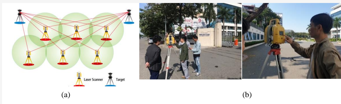
Figure 2: TLS data collection process (a) TLS reference network (b) Field data collection
