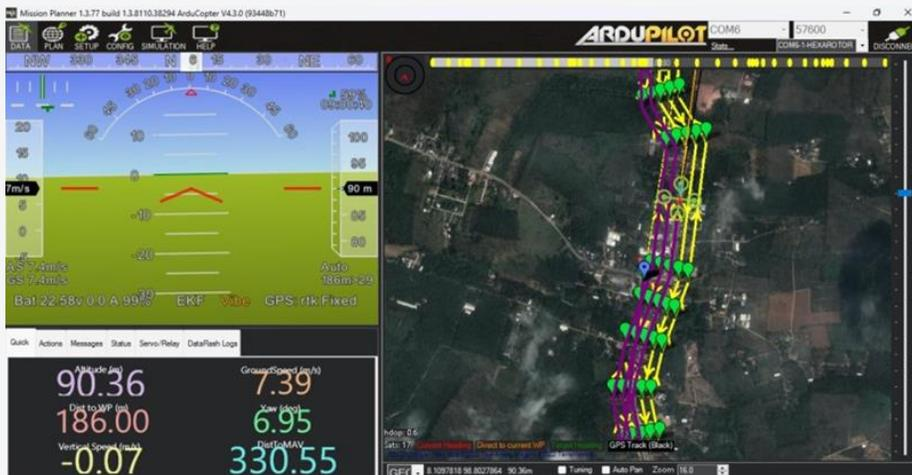
**Figure 5:** Flight plan in mission planner software
