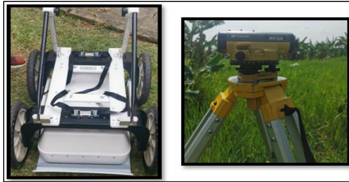
Figure 7: Equipment used in field data collection; (a) GPR equipment and (b) Auto Level
