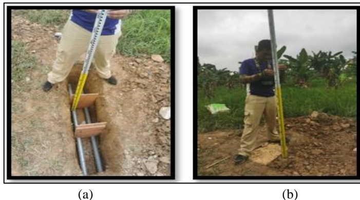
Figure 8: Levelling technique; (a) Before and (b) After buried object
