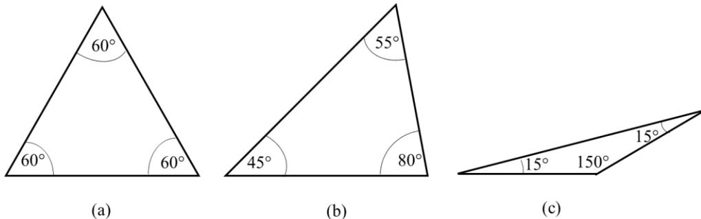
Figure 6: Definitions for the defined triangle shapes (a) an ideal-conditioned (b) well-conditioned (c) ill-conditioned
