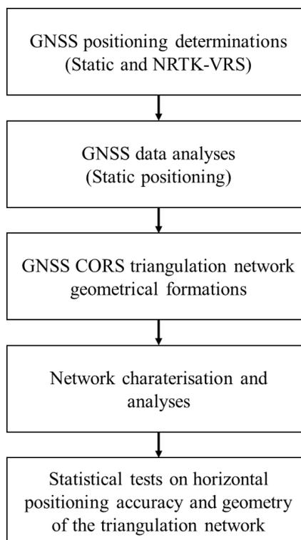
Figure 3: Computation steps on positioning performance analyses
