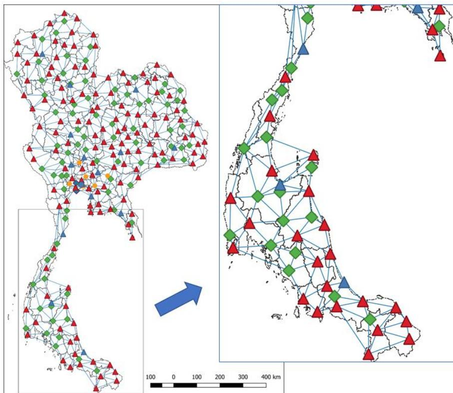
Figure 2: Illustrations on the triangulation network of GNSS CORS in western and southern Thailand
