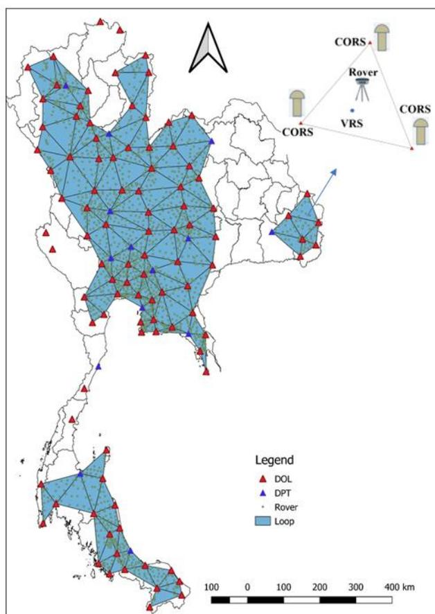
Figure 4: Locations and distributions of measured and tested marker points with their corresponding GNSS CORS network, as of June 2018
