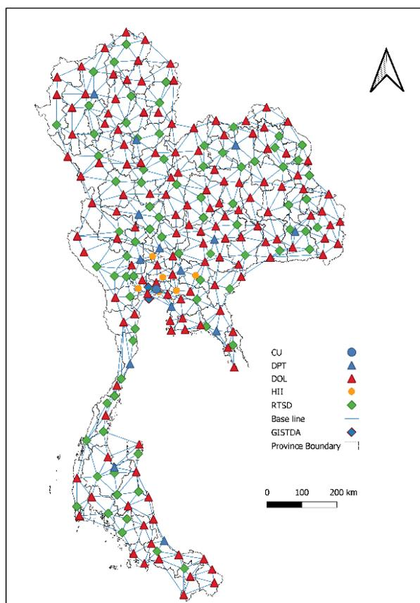
Figure 1: Geographical distributions of GNSS CORS and their triangulation networks providing NRTK-VRS GNSS positioning services
