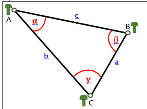
Figure 5: GNSS CORS baselines and their related angles in trigonometry
