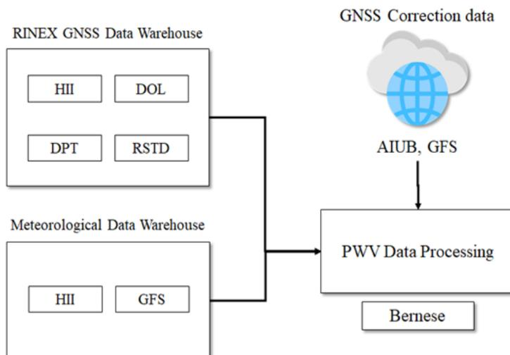
Figure 1: Near real-time PWV estimation system component
