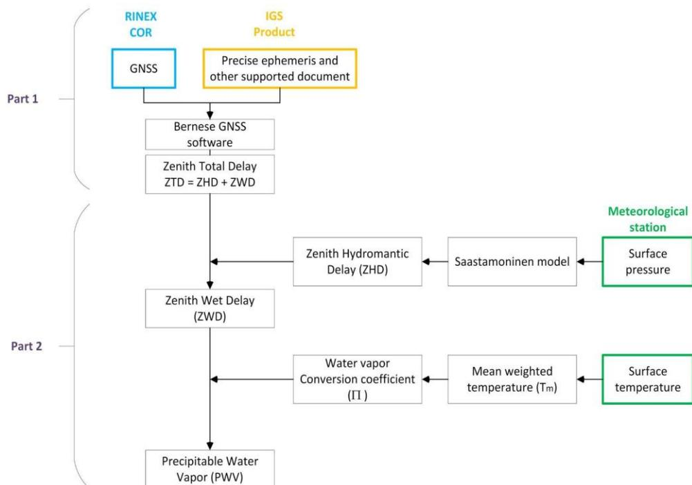
Figure 3: PWV data processing flow
