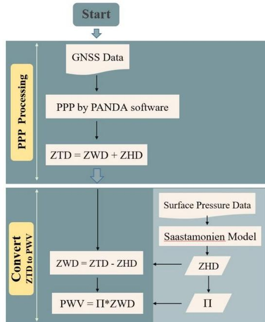
Figure 2: Data Processing from Tropospheric Delay to PWV (modified from Trakolkul and Satirapod, 2020)
