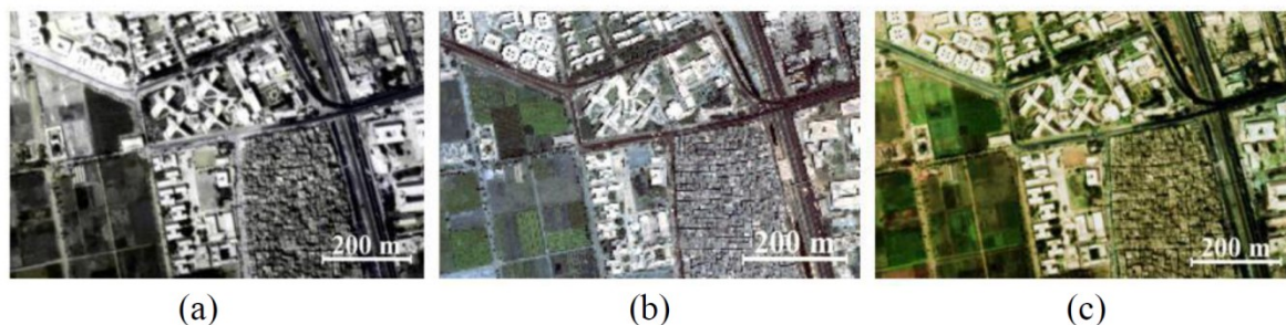
Figure 5: Results of applying the proposed pansharpening approach: (a) PAN aerial image; (b) MS IKONOS image; (c) the pan-sharpened image by the proposed approach
