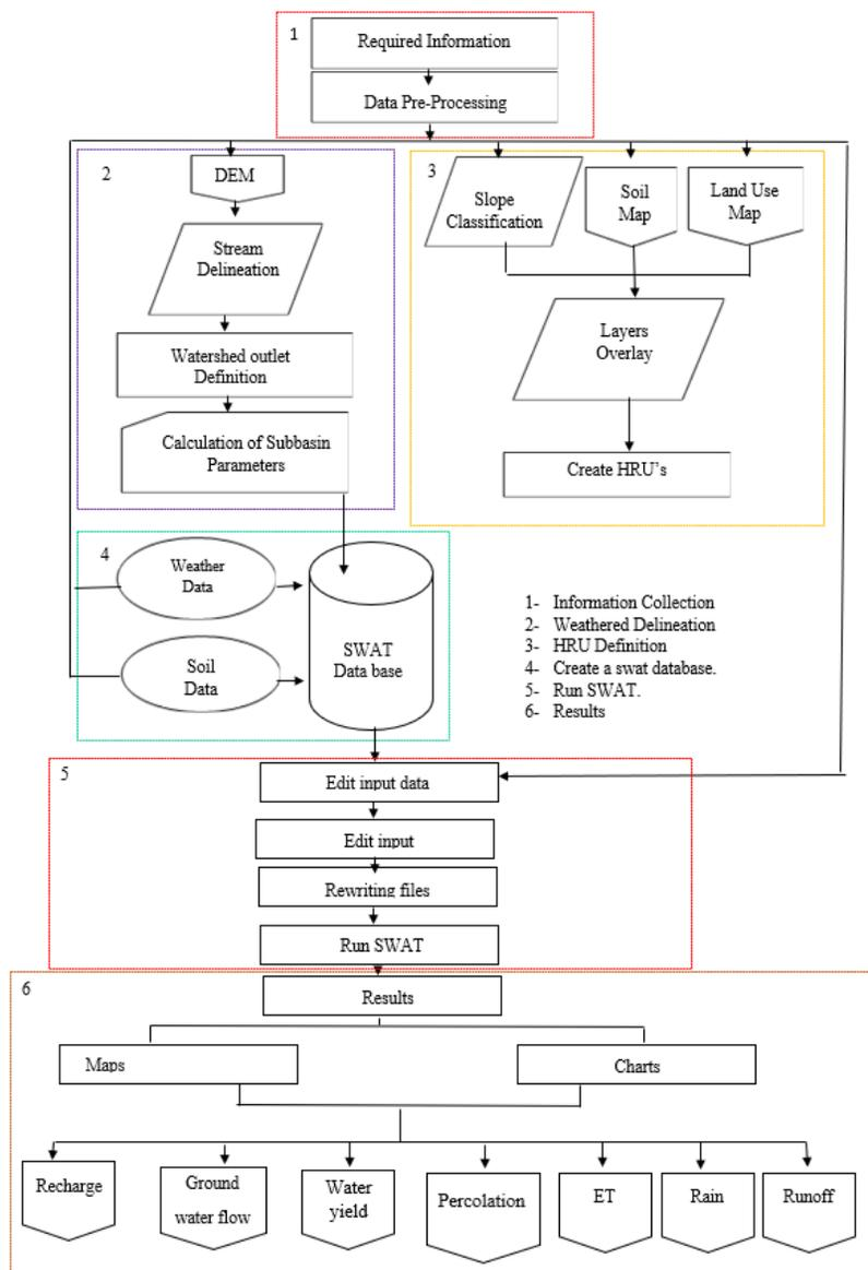
Figure 2: Representation of the steps of the Soil and Water Assessment Tool (SWAT)
