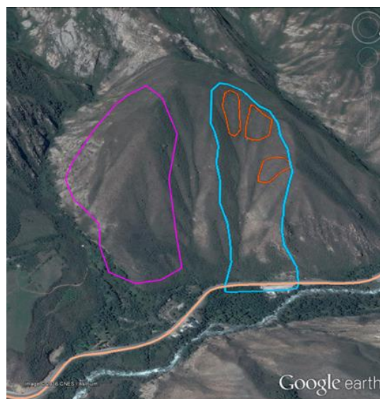
Figure 6: Hazard mapping on local scale: Verification and adaption of the catchments in the cadastre (pink), blue are the final catchments with the hazard line close to the road and the main release areas (orange)
