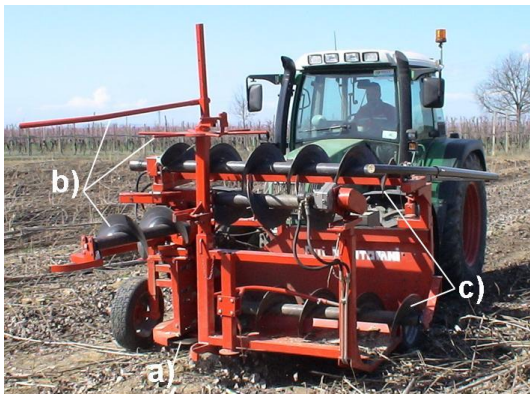
Figure 2. Specifications of the cutting (a), conveyor (b), and transporting of the machine (c)
