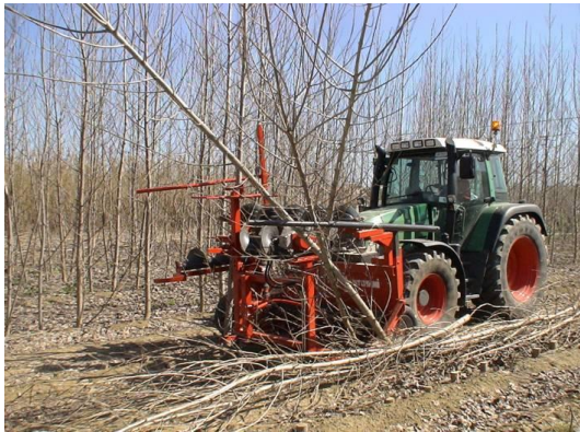
Figure 1. Mantovani cutting-aligner machine during poplar harvesting
