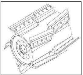
Figure 3. CRA-ING rotor mounted on Class Jaguar 890
