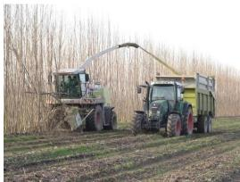
Figure 2. Class Jaguar 890 equipped with CRA-ING rotor during poplar harvesting
