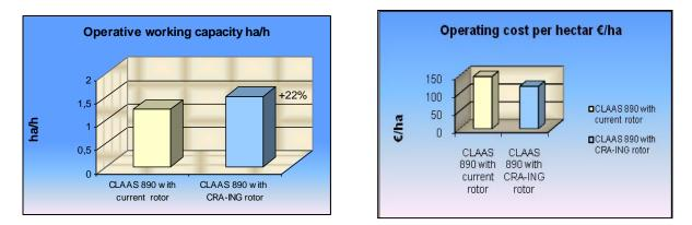
Figure 7. Class Jaguar equipped with current and rotor CRA-ING: operative working capacity and operating costs. Results obtained by harvesting simulation in the mentioned field
