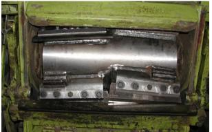
Figure 4. Ten fix knives as well slots to better fix the position on the knife holder are distinctly visible in the CRA-ING rotor
