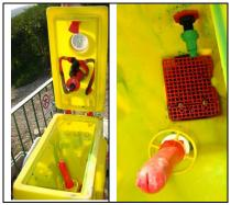
Figure 4. Chemical induction hoppers with pressure rinsing nozzles.
