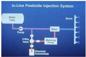
Figure 3. Schematics of an in-line pesticide injection system.
