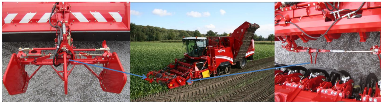
Figure 1: Sugar beet harvester MAXTRON 620 (middle), mechanical solutions for row navigation in zoom – leaves senses system (left), sugar beet head senses system (right)
