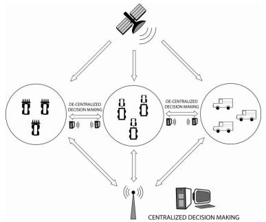
Figure 4. Basic architecture of an agricultural fleet management system
