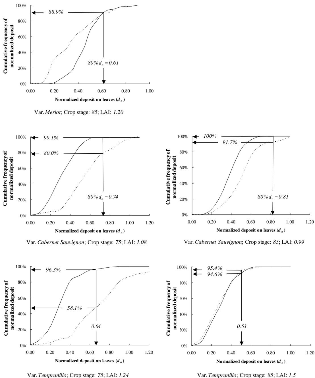
Figure 3. Cumulative frequency of normalized deposit on total leaf samples and cumulative number of samples below 80% of theoretical normalized deposit. Results for conventional application (—) and proportional according sensors measurements (-----)
