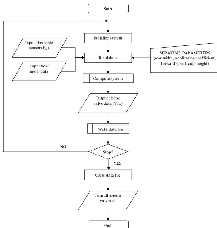
Figure 2. Flow chart of the whole electronic system for variable application
