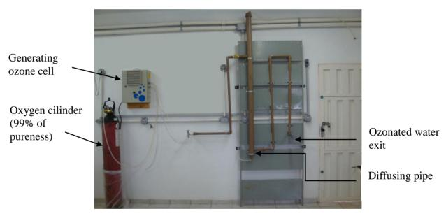
Figure 1. Equipment for production of ozonated water.
