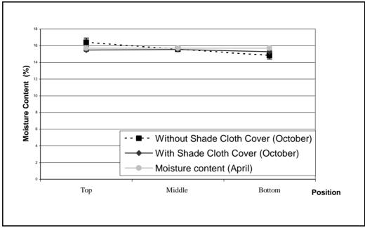
The stratification observed in the part without SCC was not observed in the part with SCC.
