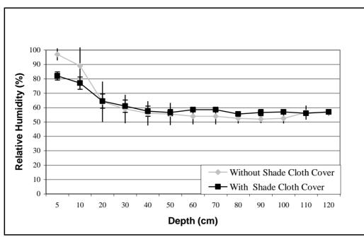
Figure 15. Relative humidity of the bulk atmosphere (variety A-3770 RG).
