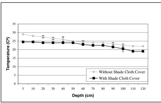
Figure 12. Grain temperature recorded at different depths within the grain mass (variety A-4910 RG).
