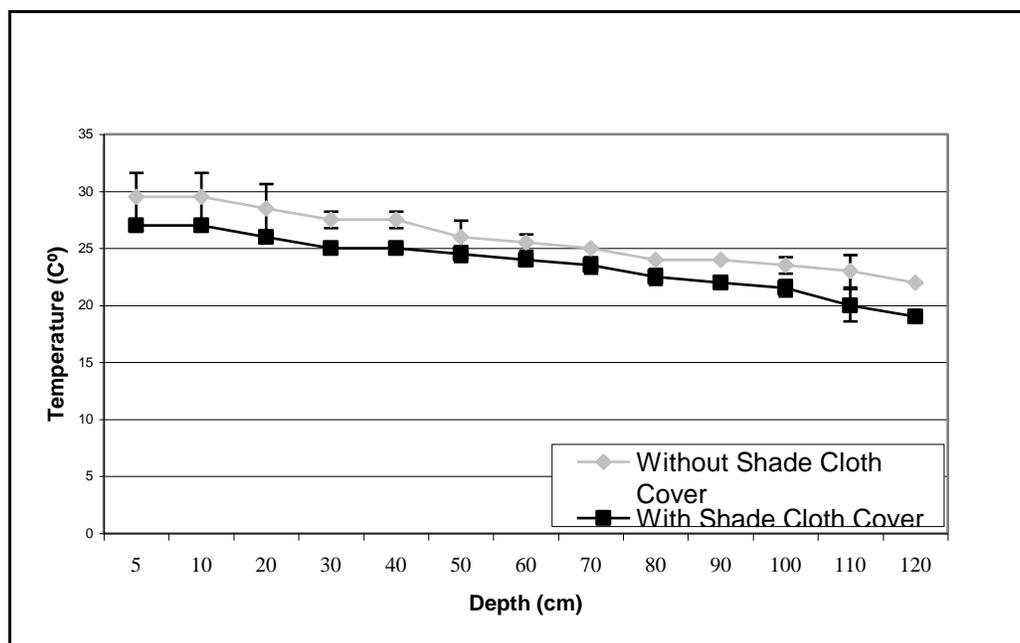
Figure 11. Grain temperature recorded at different depths within the grain mass (variety A-3770 RG).
