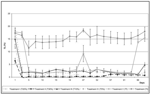
Figure 1. Oxygen concentration in the intergranular atmosphere throughout the assay.
