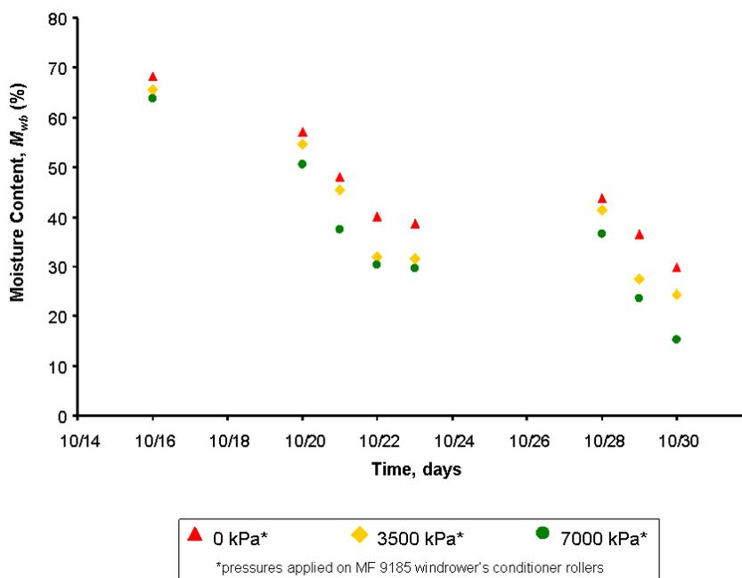
Figure 2. Sorghum moisture content for different disc header pressures for all sampled days
