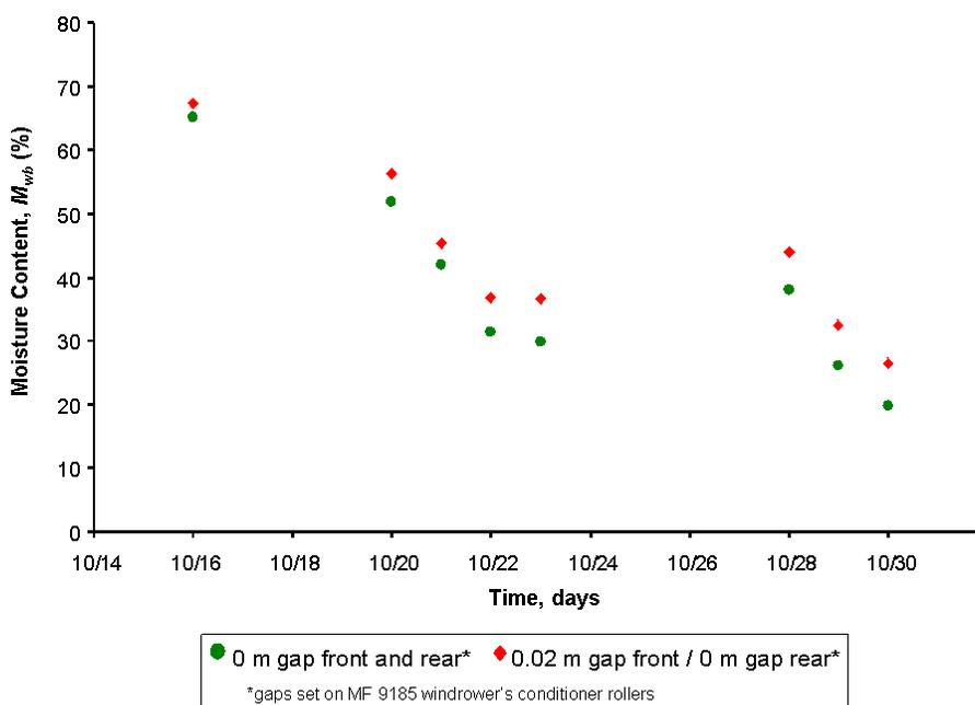
Figure 3. Sorghum moisture content for different disc header gaps in all sampled days
