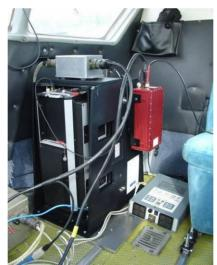
Figure 2. The installed spectral camera with red color OxTS RT3003 GPS/INS unit
