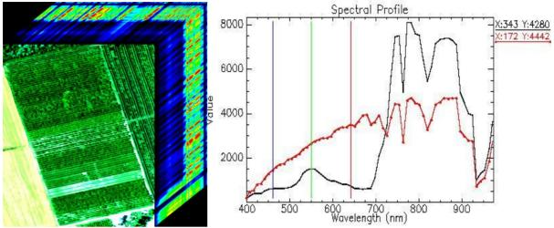
Figure 3. The 3D data cube made from 69 VIS-NIR channels and spectral reflectance curves of pixels
